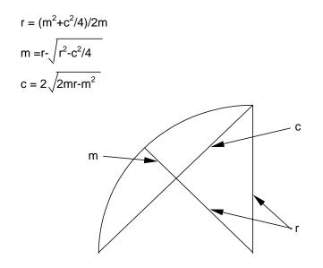
There is not a linear relationship when comparing camber measurements of different length samples. For example, if camber is measured as 1mm in 250mm, the same piece of tape that is 750mm long would not measure a camber of 3mm, but rather 9mm (the square of the multiplier).
