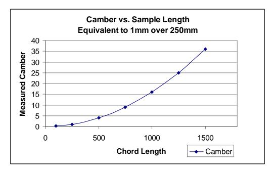
The following is a pictorial representation of the camber measurement of an arc with different chord lengths. The radius of the arc is constant, but as the chord length grows, the measured camber grows at a faster rate. Doubling the chord length increases the camber measurement by 4 times (2 squared)
